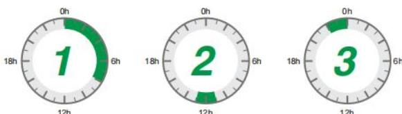
With 3 definable periods, the user can freely set the mains charging/carrying time within the range of 00:00 to 23:59. During the time period set by the user, if PV energy is available, PV energy will be used first, and if PV energy is not available or insufficient, utility energy will be used as a supplement.
